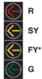
Figure 10 Typical Arrangement of Separate Signal Faces with FYA for Protected/Permissive Mode and Protected Only Mode Left Turns (Source MUTCD, Dated May 2012)
